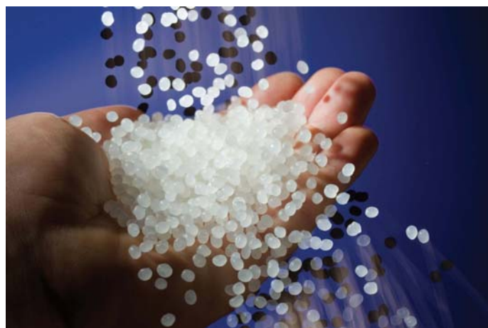
Polysole XD, an all-natural, biodegradable plastic that could find use in interior parts, comes as meltable pellets.
