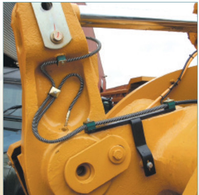
Protected heavy duty flexibles fitted to a CAT loading shovel
